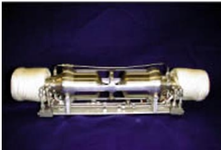
Figure 19. Stirling engine powered by a radio isotope heat source, NASA Glenn Research Center.
